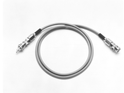
Agilent 16117E low noise test lead Male-triaxial to male-triaxial connectors. One meter cable. One female-triaxial connector included. For 4349B only.
